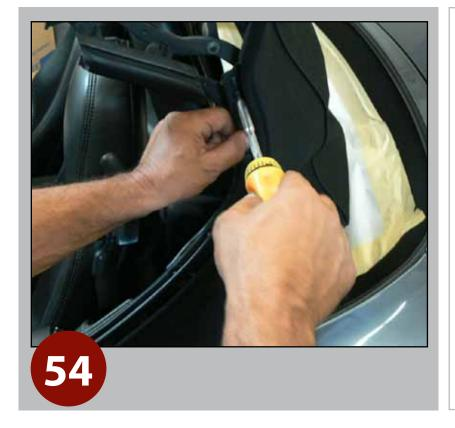
Secure the front header rail to the frame.
