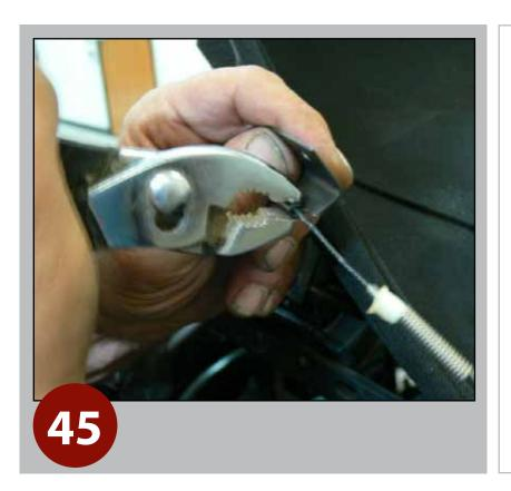
Then, connect the new "L" shaped brackets that came with your new convertible top to the existing side tension cables.
