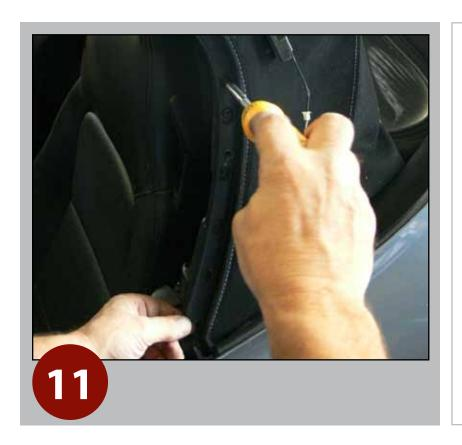
Remove the screws under the side quarter rubbers to detach the brackets.
