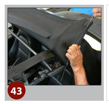
Now you can insert your existing tension cable removed earlier through the top sleeve.
