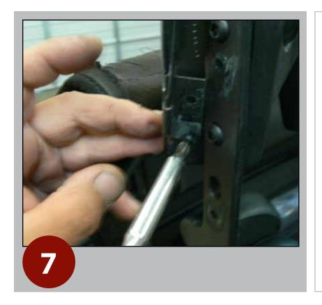
Remove the side "L" shaped bracket to free the cable.
