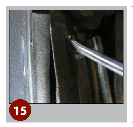
Cut rivets located at the end of the rear tacking strip.
