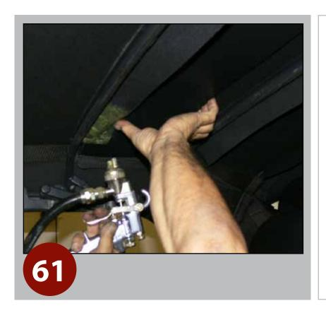
Attach all three top listers by using contact cement adhesive.
