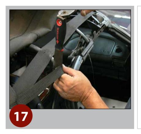
Cut or drill rivet to remove elastic straps from second bow.
