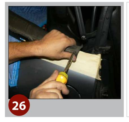
Remove the end screws and there are some staples here that will need to remove as well.
