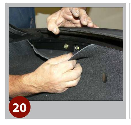
Pull away the well lining to access the bolt nuts underneath.
