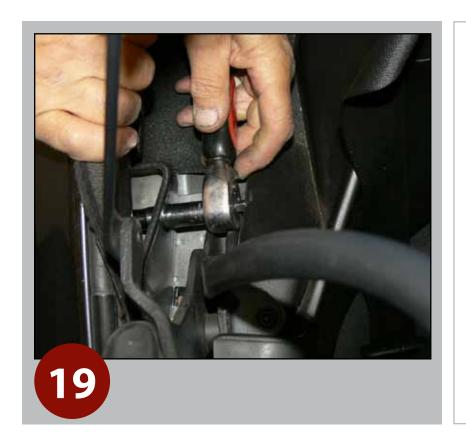
With your 5/32" socket wrench, start to remove the tacking bow bolt nuts at the quarters.
