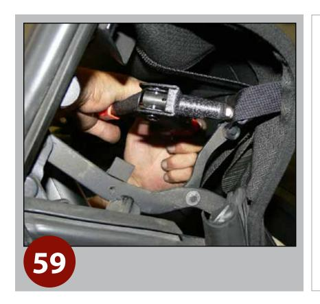
Use rivets to secure in place.
