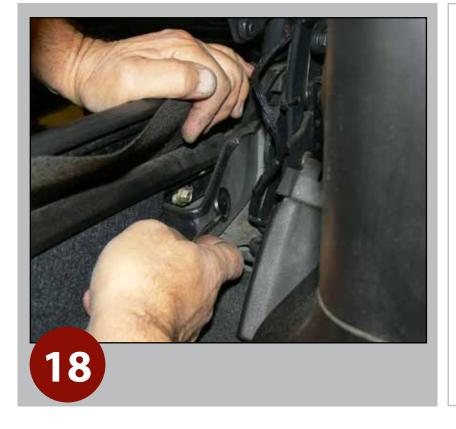
Remove the top well quarter plugs to access tacking bow bolt nuts.
