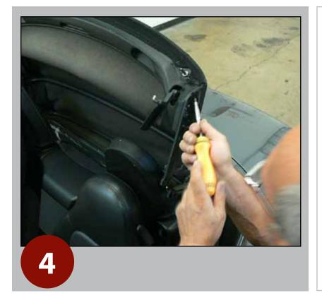
Once the rubbers are out of the way, you can begin removing the screws as shown.
