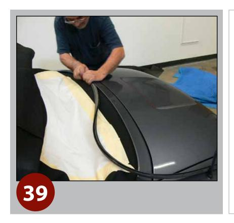
Re-install the rubber strip to the edge of the top well.
