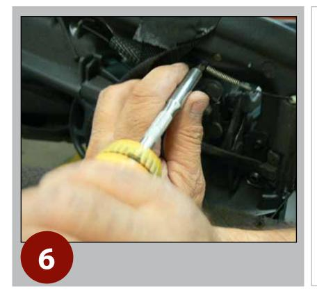
The next step is to remove the tension side straps. Begin by removing the tension cable screw.
