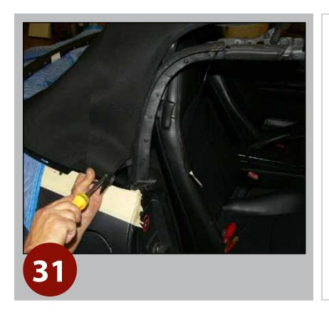
Begin by attaching the top, using screws, to the tacking bow.
