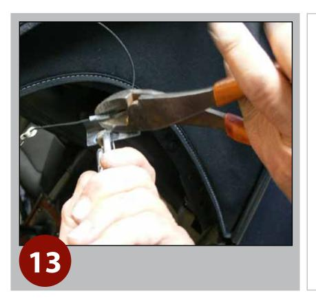
Separate the "L" shaped bracket from the cable and pull out the cable from the sleeve on the side of the existing convertible top.
