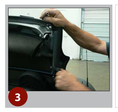
Next, you will need to remove the front side rubbers to access additional screws to be removed.
