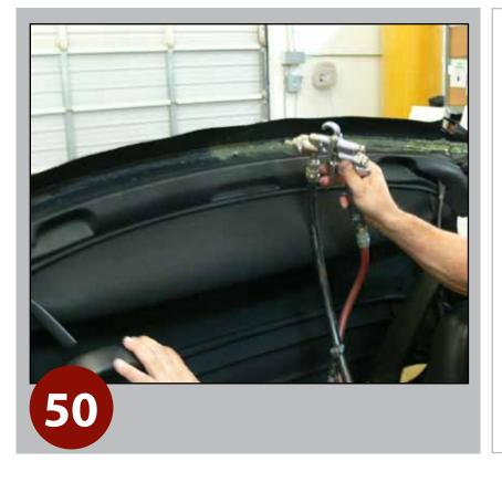
Using a spray contact cement adhesive, attache the new convertible top to the front header.
