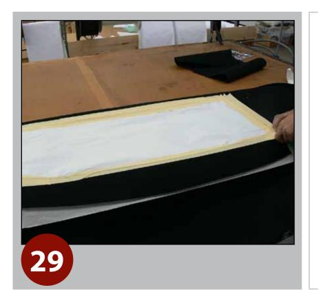
View of the plastic window section fully protected so it does not get scratched during the installation process. Use a masking tape that will come off easily and cleanly.
