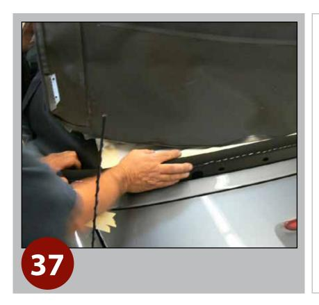
After you have completed the stapling, drop in the tacking bow into the top well and position it to the body bolts.
