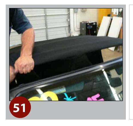
Press firmly to stretch the top to the header bow. Work with the top nearly closed to judge the tightness of the new top.
