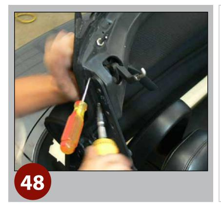
Secure the front side of the top and quarters to the frame, but do not install the screws yet.
