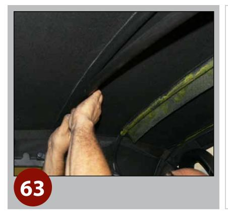
Complete attaching the "C" channel rails, then take off the plastic window protection to finish the project.
