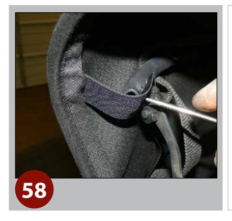
Position top side straps to frame arm. These are the elastic tesion straps that assist in pulling the top material inward as you are opening it.
