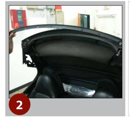
Once the screws have been removed, detach the header rail.
