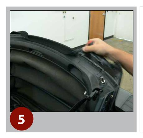
Start to peel back the front edge of the top.
